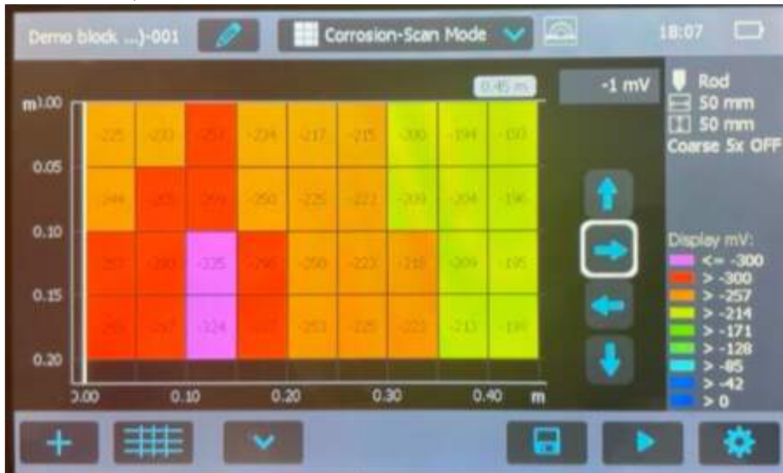
Corrosion likelihood using Profometer Corrosion
