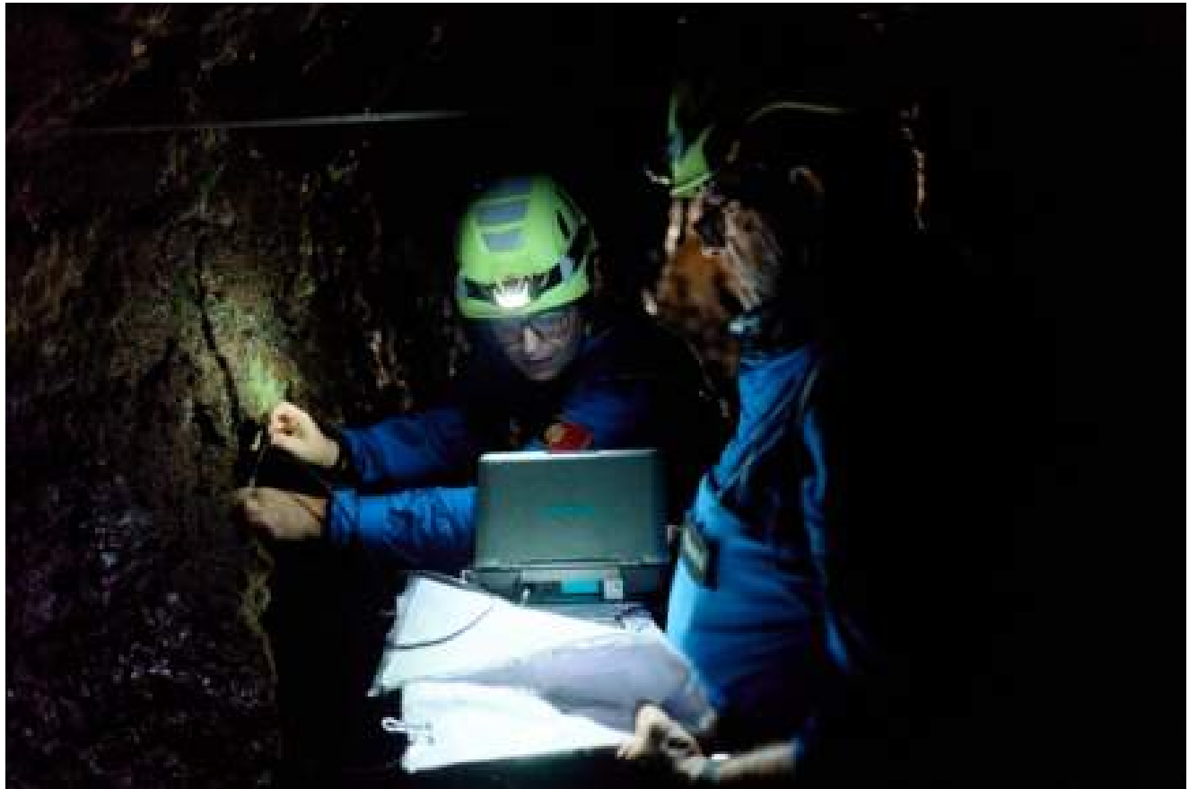
Ana Pires takes hardness measurements inside the lava tube with the Equotip portable hardness tester.
