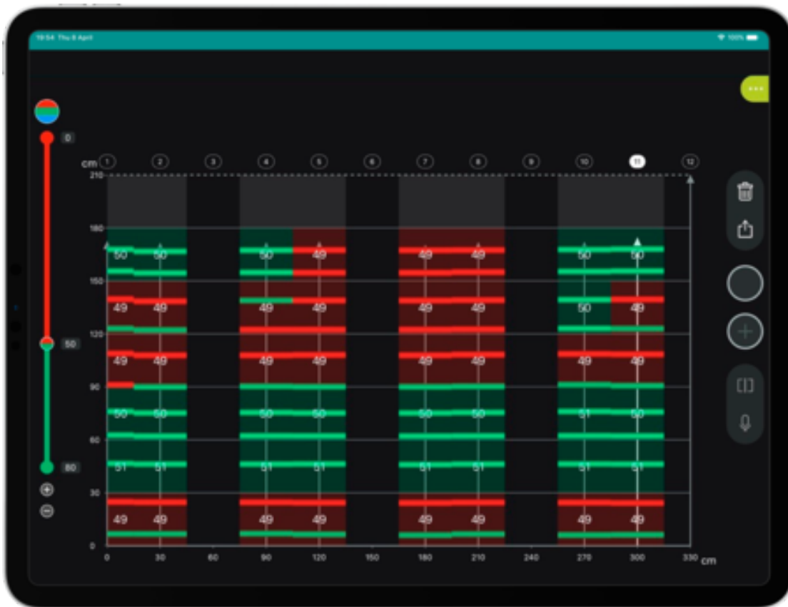
Scanning column's stirrups in vertical scanning direction
