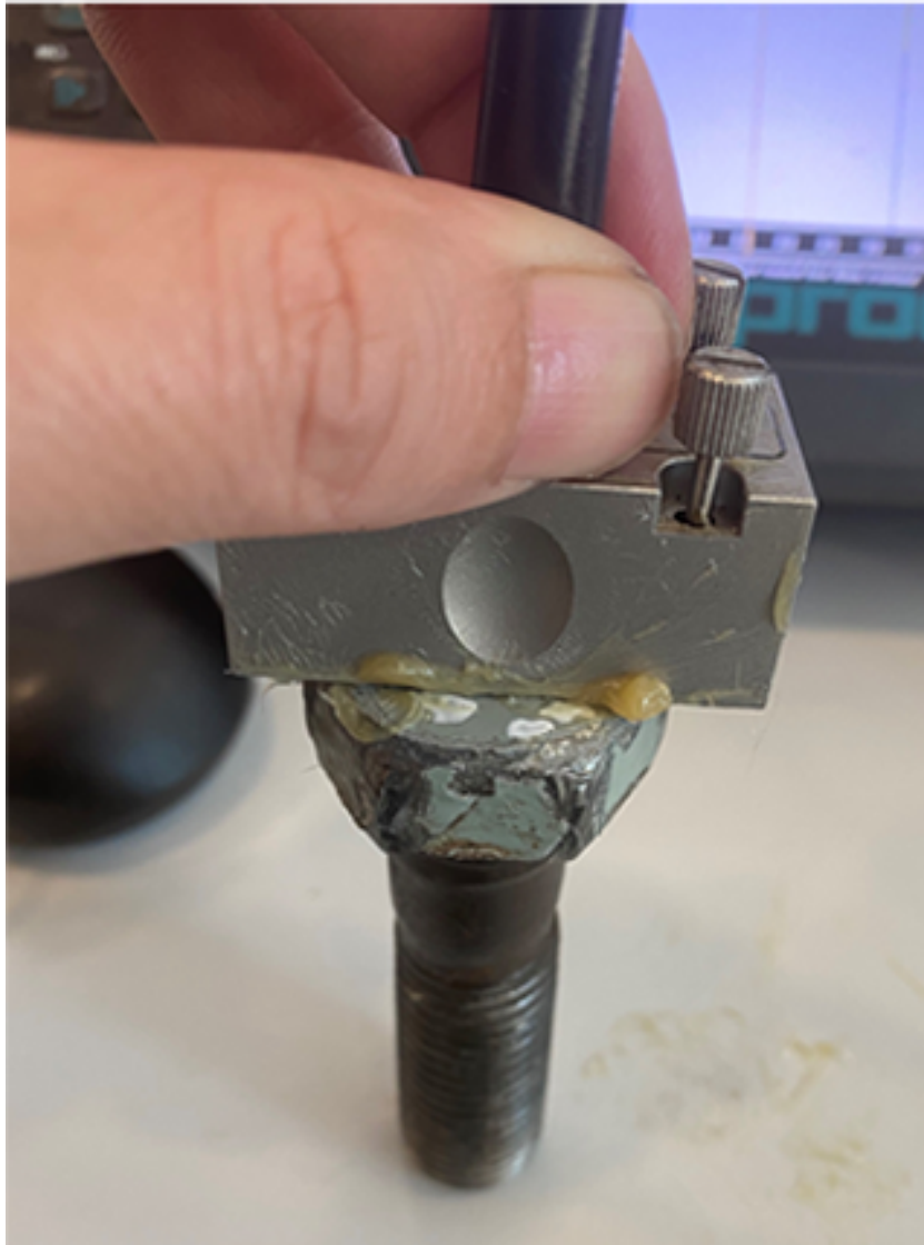
Phased array probe being held on a bolt. The bolt is ex-situ for the 'proof of concept' project but an identical testing method can be used with the bolt in-situ
