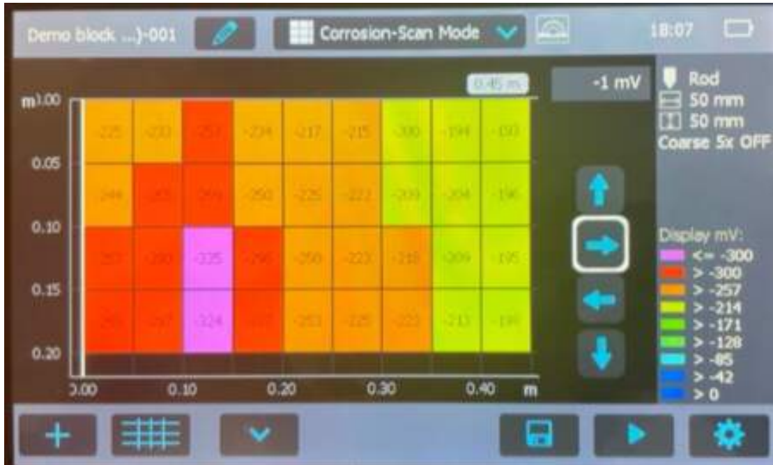
Corrosion likelihood using Profometer Corrosion
