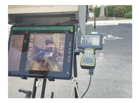
Using a Robotic Total Station with Screening Eagle's 'free path' function is of great benefit to subsurface utility engineers and surveyors. A map of the subsurface is generated immediately without the need for multiple processing steps or further work off-site. The surveying workflow is streamlined and fully achievable by one person.
