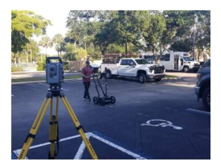
The Proceq GS8000 boasts a unique 'free path' function which allows the surveyor to walk freely, unconstrained by a grid. The resulting heatmap of the subsurface is plotted on a map in real-time, at the desired depth range.
