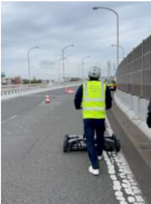
Figure 2 and Figure 3 show the GS9000 system operating on the bridge deck
