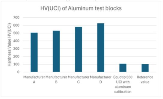
To ensure accurate measurements, special calibrations accounting for different Young's moduli are required. Manufacturers often provide these, or users can create their own through external calibration.
