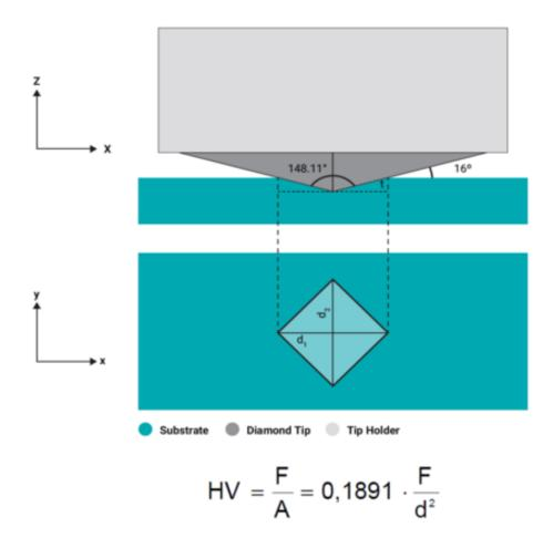
The **UCI method** uses the same diamond indenter but mounted on a vibrating rod that resonates at an ultrasonic frequency. When the diamond indenter is pressed into the material, the surface contact between the indentation and diamond alters the resonating frequency. The larger the indentation, the greater the frequency change. Rather than measuring the diagonal of the indentation optically, the UCI method uses the frequency shift to instantly calculate the hardness value.
