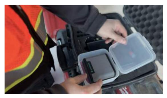
Furthermore, the new battery Li-ion gives new flexibility when charging your GP8800. Now, you can easily recharge the battery from the car, your laptop, the airport, café, or anywhere else with a USB port. With full voltage flexibility, you can recharge anywhere.
