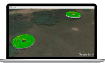
GNSS positions around the two trees, overlaid on Google Earth image. Green colour indicates an excellent GNSS correction status and yellow indicates a less good status.
