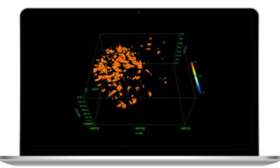
3D results displayed in GPR-SLICE. The 3D orange shapes are areas of higher reflection amplitude and they represent the architectures of tree roots, in particular the anchorage roots.
