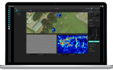
Since the data was collected with centimeter level accuracy GNSS, depth slice results could be superimposed on a geo-map. We can easily understand the distribution of tree root system within the measurement coverage. By pinpoint on the geo position we can locate what we want at actual location.
