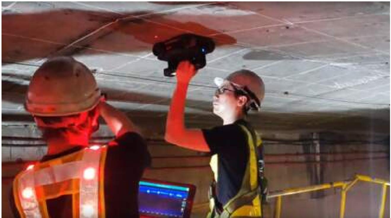
The Proceq GP8000 GPR scanning thick concrete
