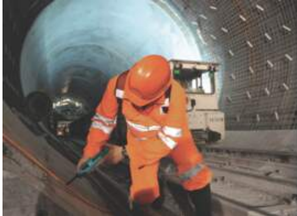
Next generation rebound hammer for concrete, the Silver Schmidt
