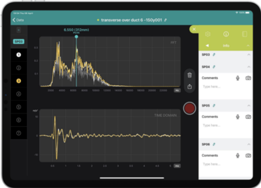
Air voiding as shown with Pundit PI8000 ultrasonic impact echo technology, taken in the same spot as the PD8050.
