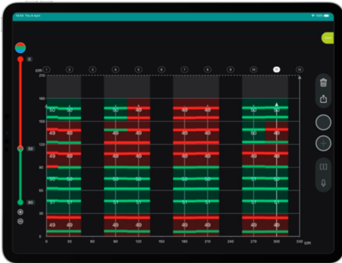
Scanning column's stirrups in vertical scanning direction
