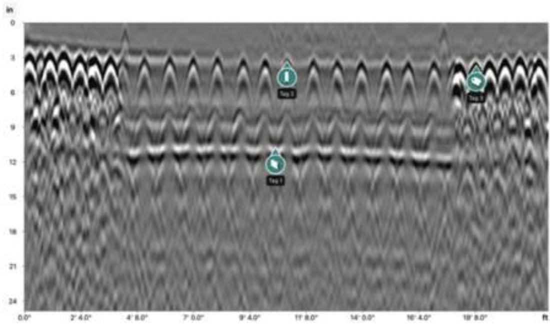
Figure 4: GPR scan across box girder width.
