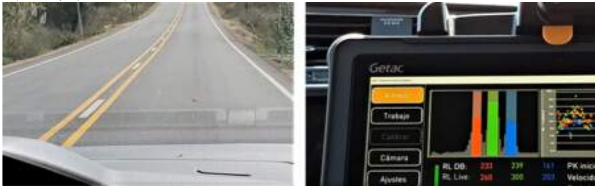
Example of a road with triple road markings (left) and the results as seen live on ZDR6020 software (right).
