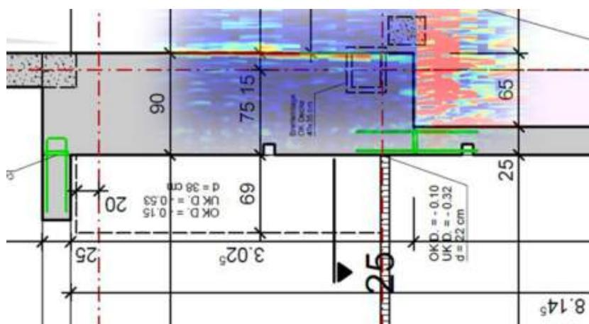
Screening Eagle Technology’s portable ultrasonic imaging device, [Pundit PD8000](#), is used to generate 2D and 3D images of concrete structures up to 2m thick. The images are generated immediately on site. The high signal-to-noise ratio and advanced imaging algorithms produce high quality images from which defects can be quickly identified and tagged. Views and maps are also instantly available in the field.
