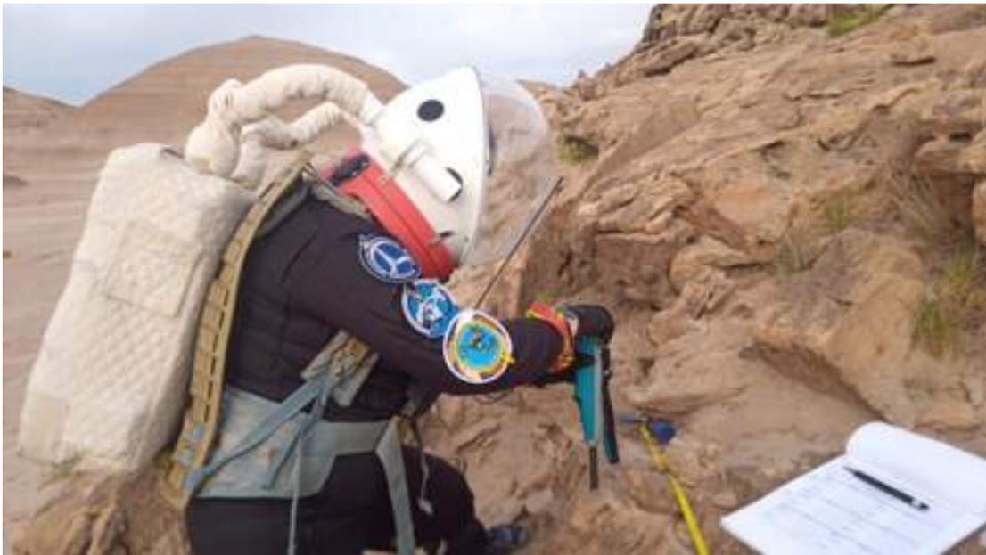
The [Equotip hardness tester](#) is mainly used to evaluate metal, however it is also a convenient tool to test the Unconfined Compressive Strength (UCS) of rock.
