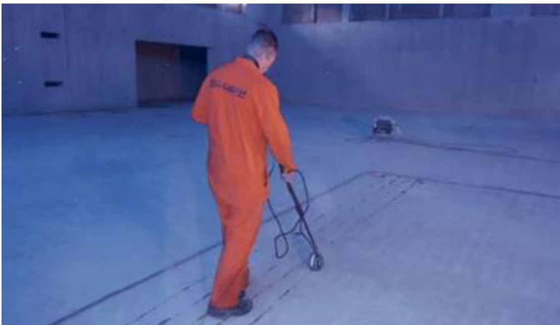
Performing half-cell potential measurements on the concrete floor with the Profometer PM8500 corrosion sensor
