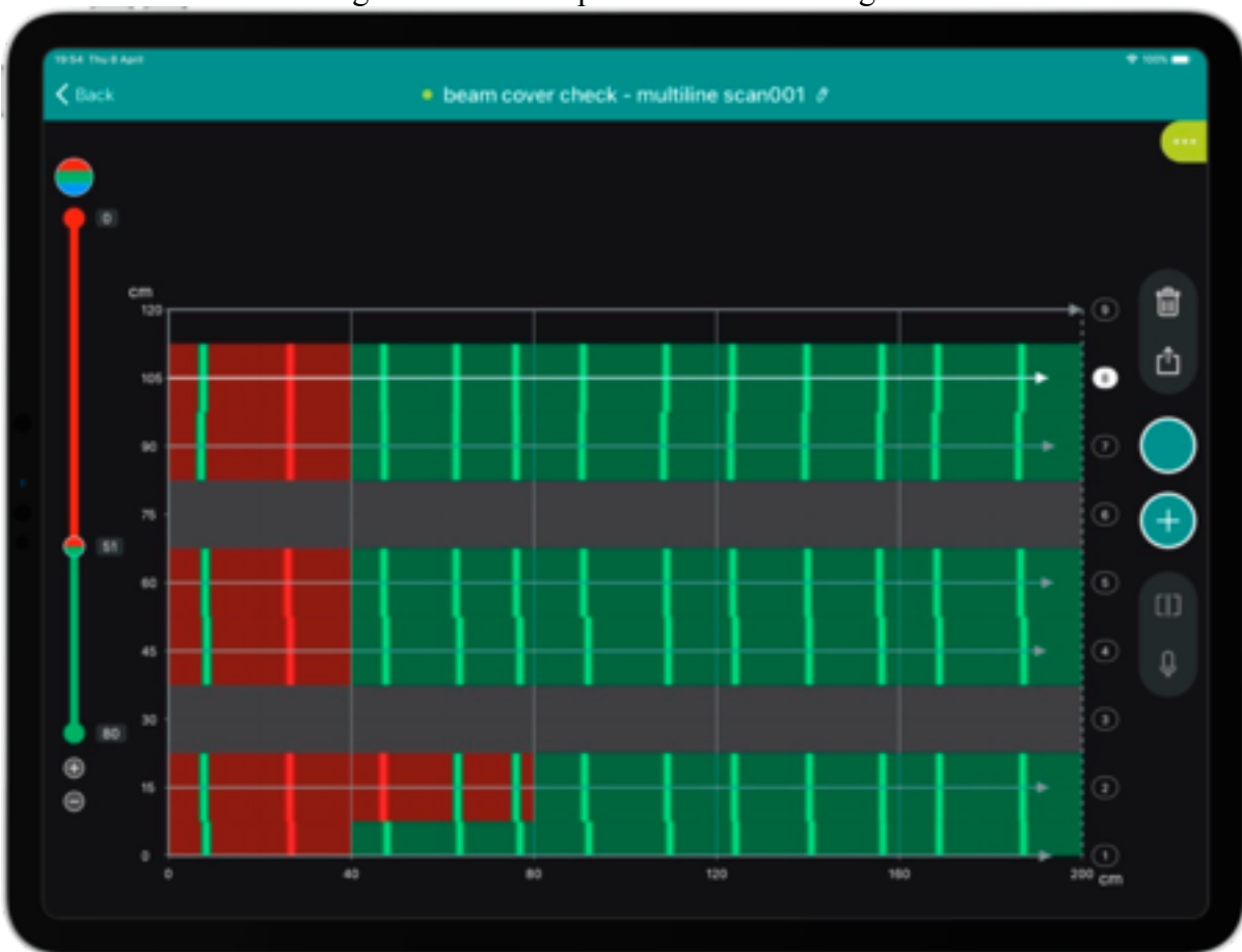
Scanning beam's stirrups in horizontal scanning direction
