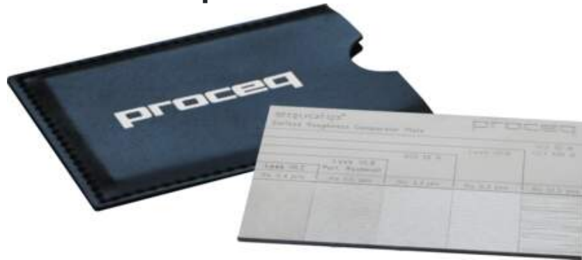
Equotip Surface Roughness Comparator
