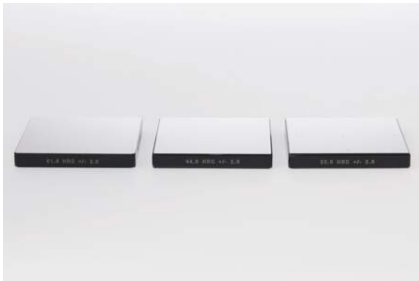
Equotip Portable Rockwell Test blocks
