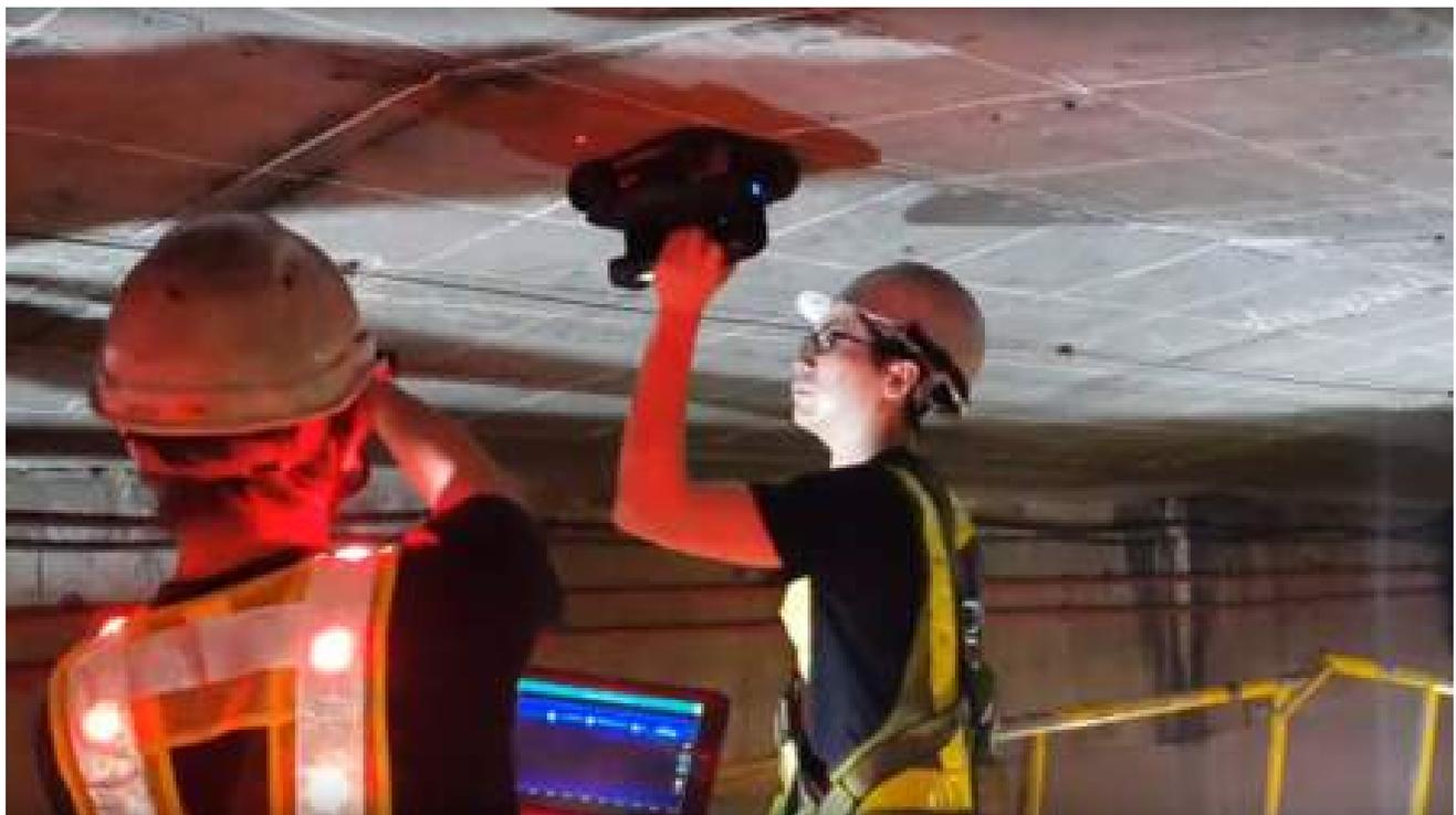
The Proceq GP8000 GPR scanning thick concrete
