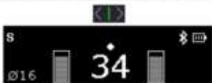
Press and hold the left key button for 2 seconds to calibrate the signal strength indicator on the reference rebar
