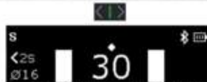
More intense signal detected means bigger object detected (Assuming same depth than standard rebar, here cover is slightly lower because of the wrong diameter setting).
