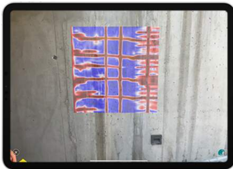
Area scan data shown on the iPad (left) and on the concrete surface (right)
