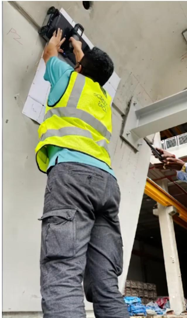
With the use of powerful data collection software, the [GP8100](#), visualizes 3D data in real-time and the results can be presented in different views, like time-slice or as Augmented Reality (AR) view on the scanned area. Embedding the 2D or 3D results on the site using AR, allows us to capture the subsurface reality as is and create an intuitive report.
