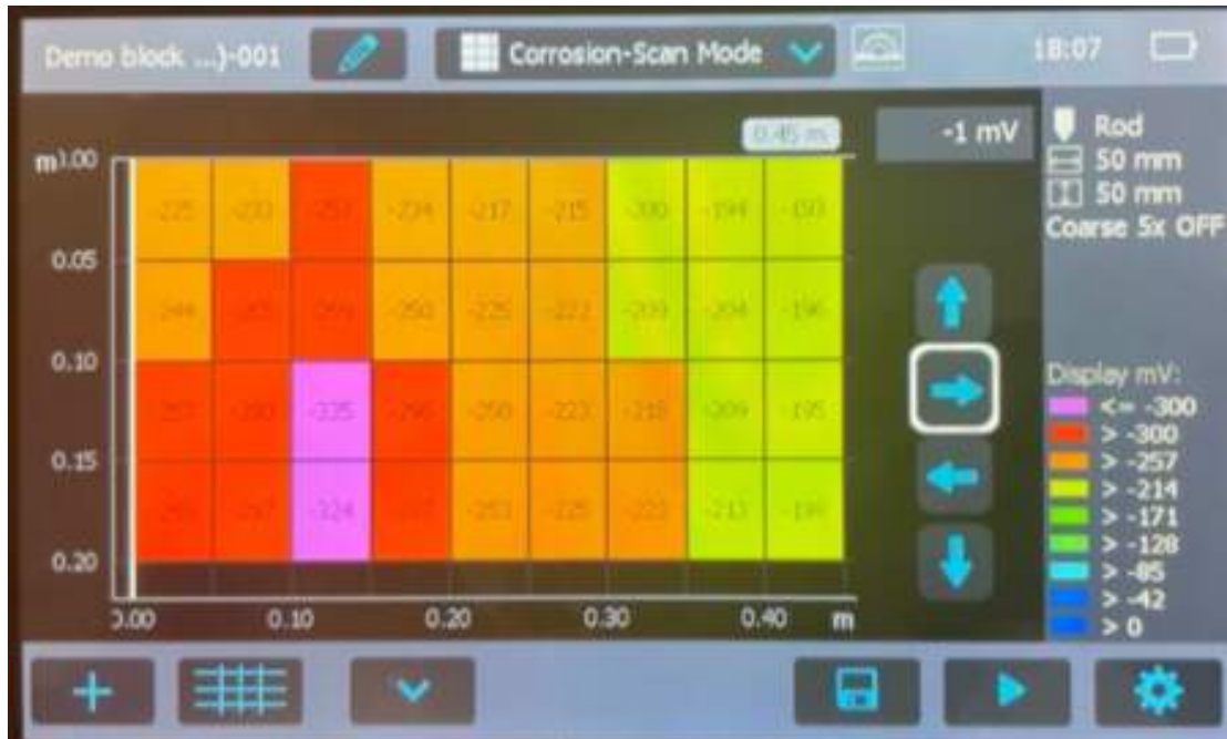
Corrosion likelihood using Profometer Corrosion
