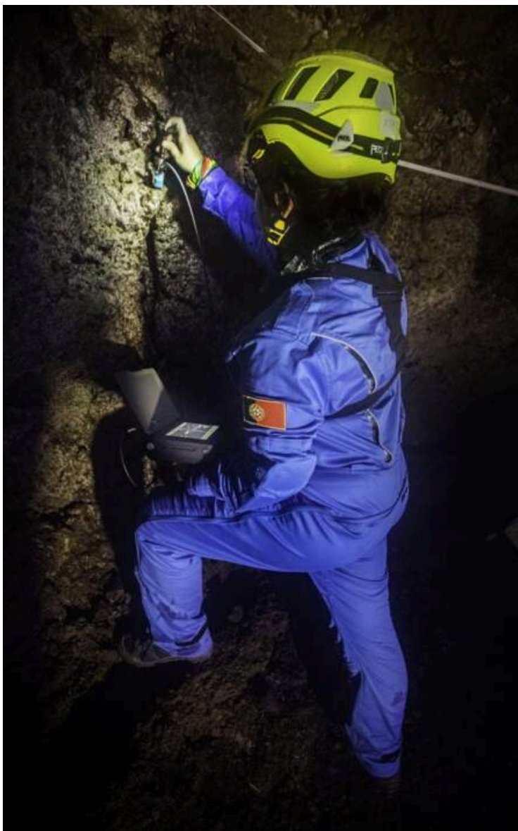
Ana Pires taking measurements with the Equotip portable hardness tester
