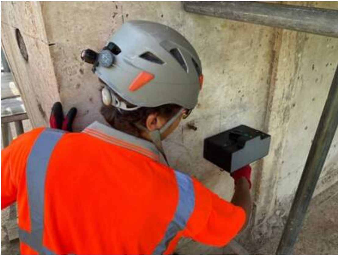
Non-destructive testing on the Huntingdon Railway Viaduct
