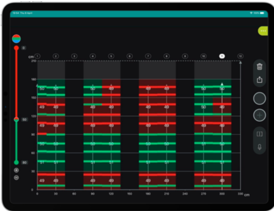
Scanning column's stirrups in vertical scanning direction
