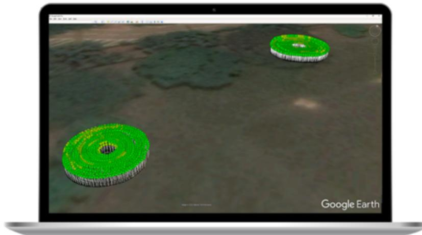
GNSS positions around the two trees, overlaid on Google Earth image. Green colour indicates an excellent GNSS correction status and yellow indicates a less good status.
