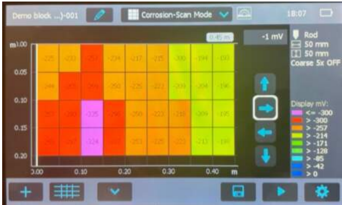
Corrosion likelihood using Profometer Corrosion
