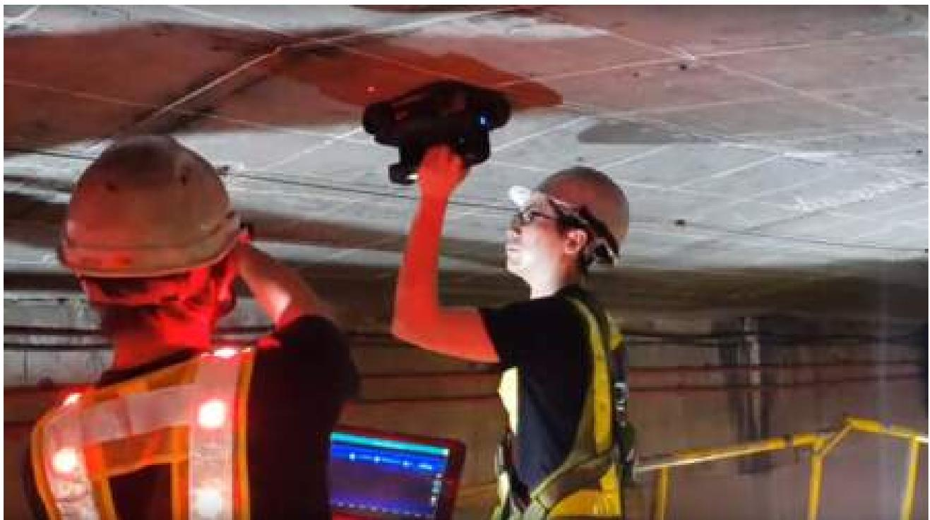
The Proceq GP8000 GPR scanning thick concrete
