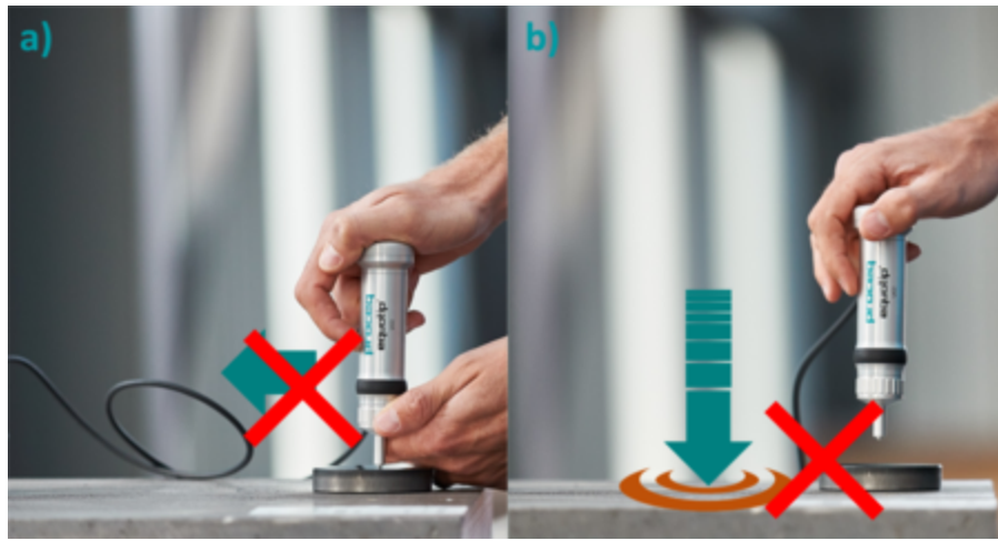
Figure.2. Schematic illustrations of potential probe applications that may lead to damage of the indenter. a) Lateral movements of the probe during the indentation. b) strong impact of the p
