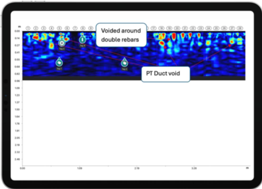
Results from the PD8050 showing localised voiding, taken over the same location as the GPR scans. Additionally the double rebars appear to have voiding around them.
