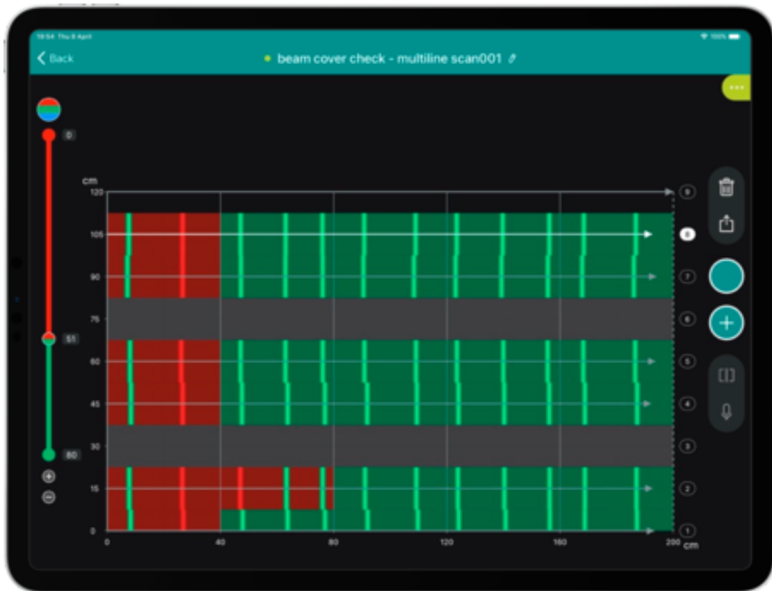
Scanning beam's stirrups in horizontal scanning direction
