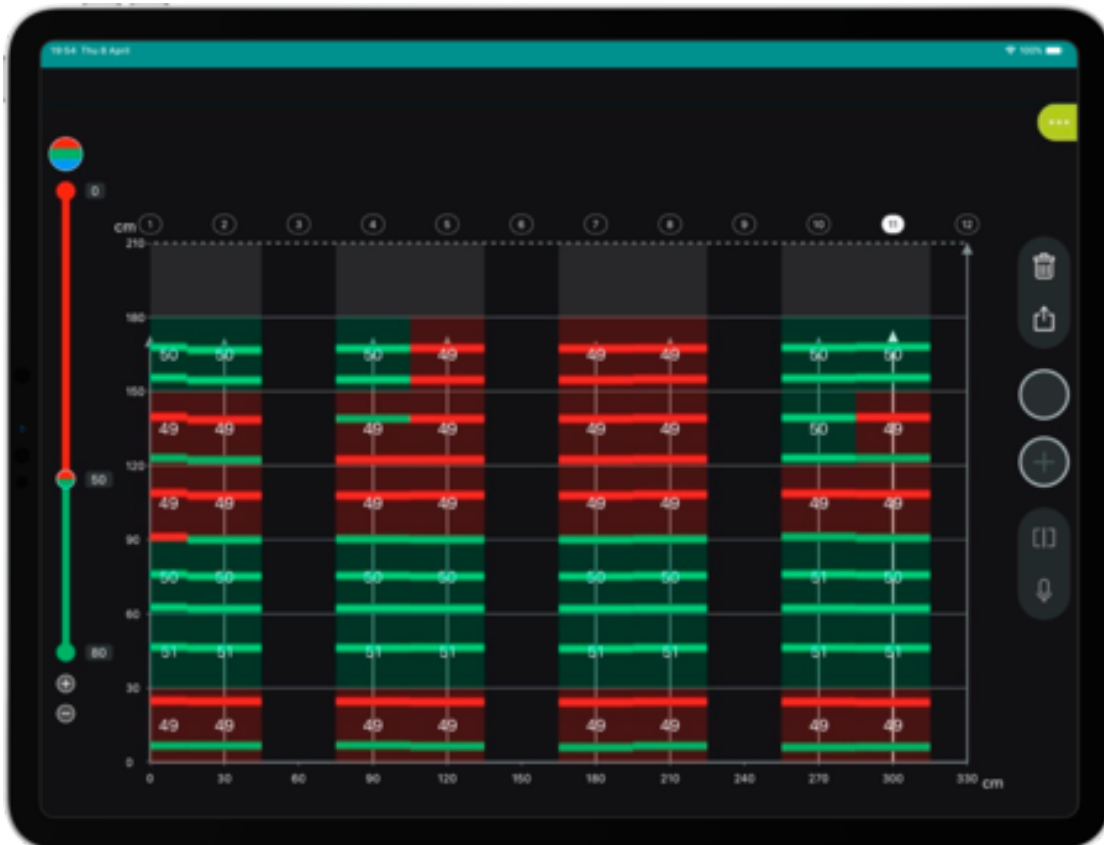
Scanning column's stirrups in vertical scanning direction
