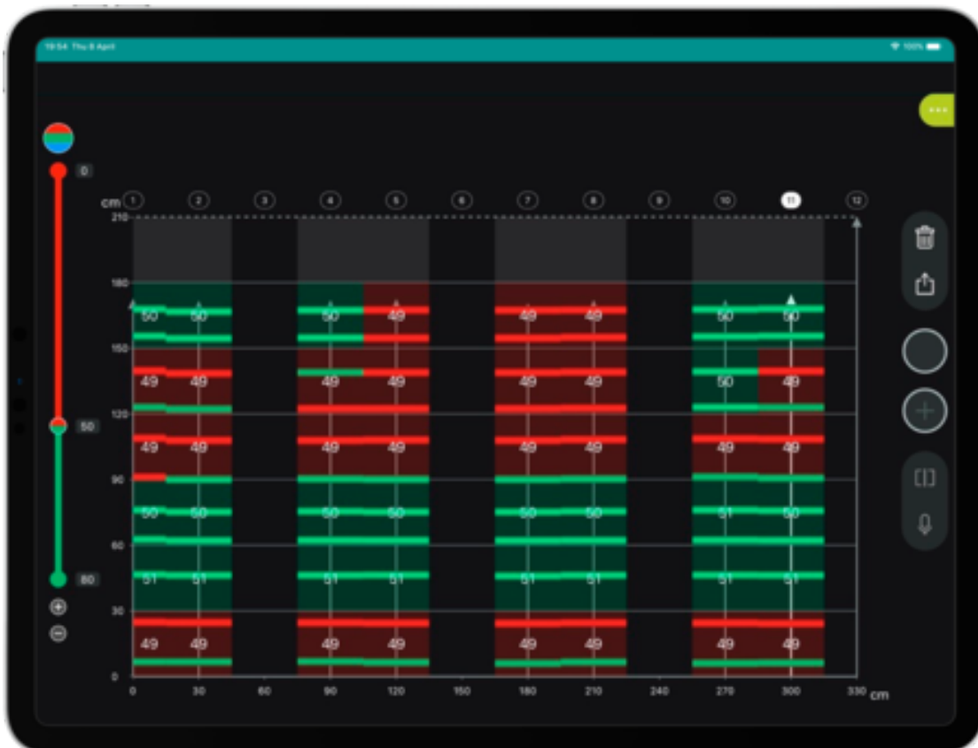
Scanning column's stirrups in vertical scanning direction
